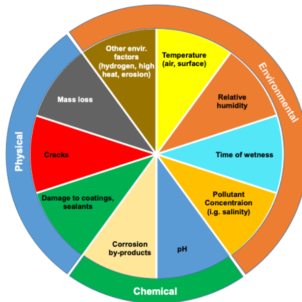
Figure 1. Corrosion matrix of physical, chemical, and environmental factors [11].
